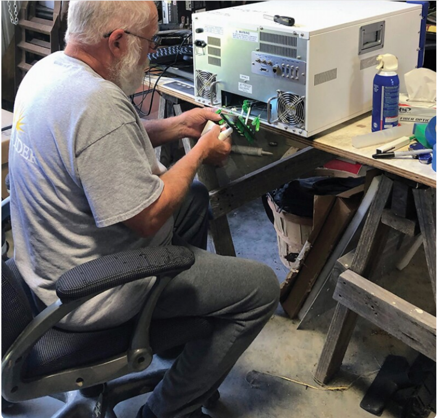
Maintaining an interrogator unit used to measure fiber-optic data. Source: Neubrex.
